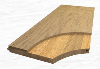
Twinface parquet floorboard is wooden flooring that occupies an intermediate niche between the solid wood parquet and engineered wood flooring. Twinface parquet flooring is a two-layer structure where the top layer consists of oak lamella and the bottom layer is the panel made from finger-jointed and glued together oak battens.
